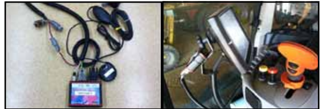
Figure 2. Vector™ CAN Case XL and Vector™ CAN GPS data logging system (left) and Vector™ system installed on a self-propelled forage harvester.
