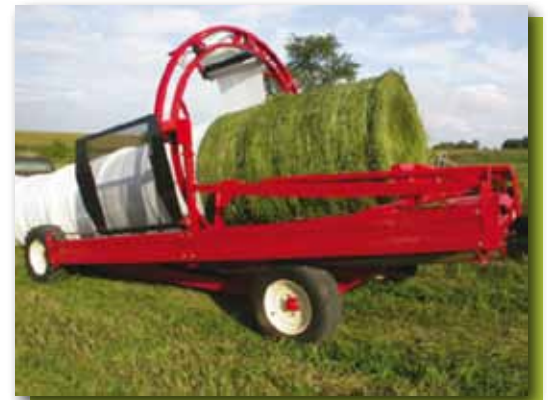
In-line or tube wrapping may be faster than individually wrapping bales.
