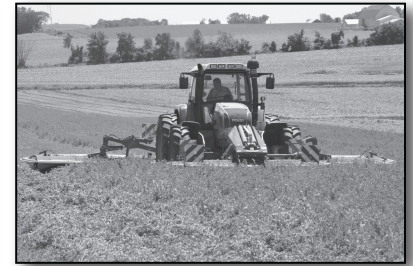
Hay is cut using a Pottinger 33' disc cutter.
