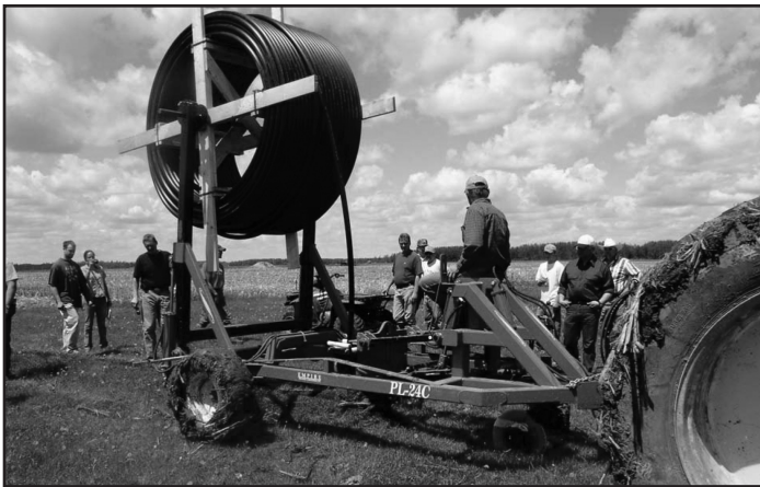
In some situations it is desirable to bury pipeline. This is set up for shallow burial of pipeline.
