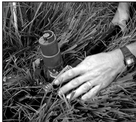
Compression fittings speed up the process of joining or disassembling pipe sections and come in a number of configurations. A quick coupler set up for portable water tanks is shown in the photo. This acts much like a hydraulic hose coupler. Flap is raised and hose fitting inserted into the flap.
